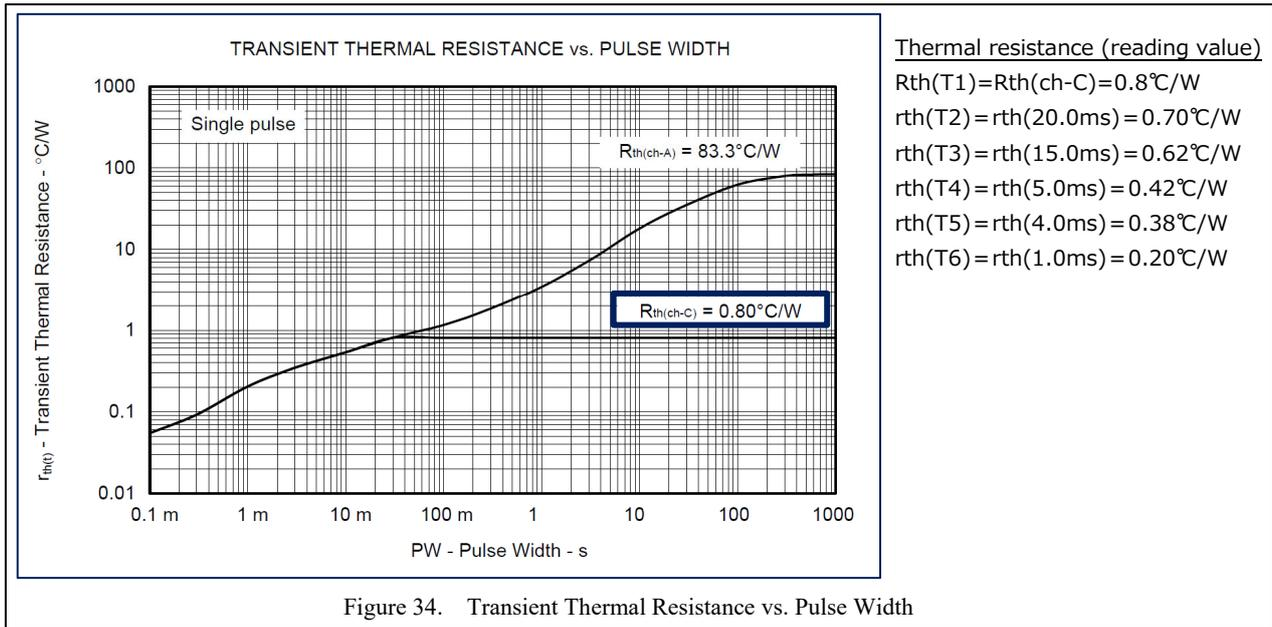
Figure 34. Transient Thermal Resistance vs. Pulse Width
