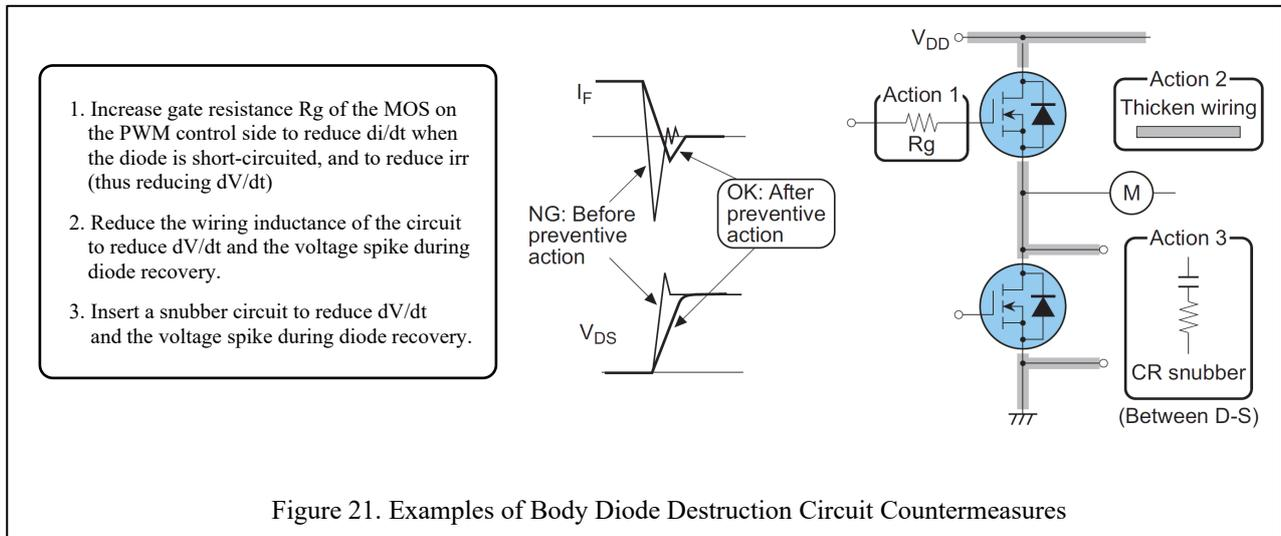
Figure 21. Examples of Body Diode Destruction Circuit Countermeasures
