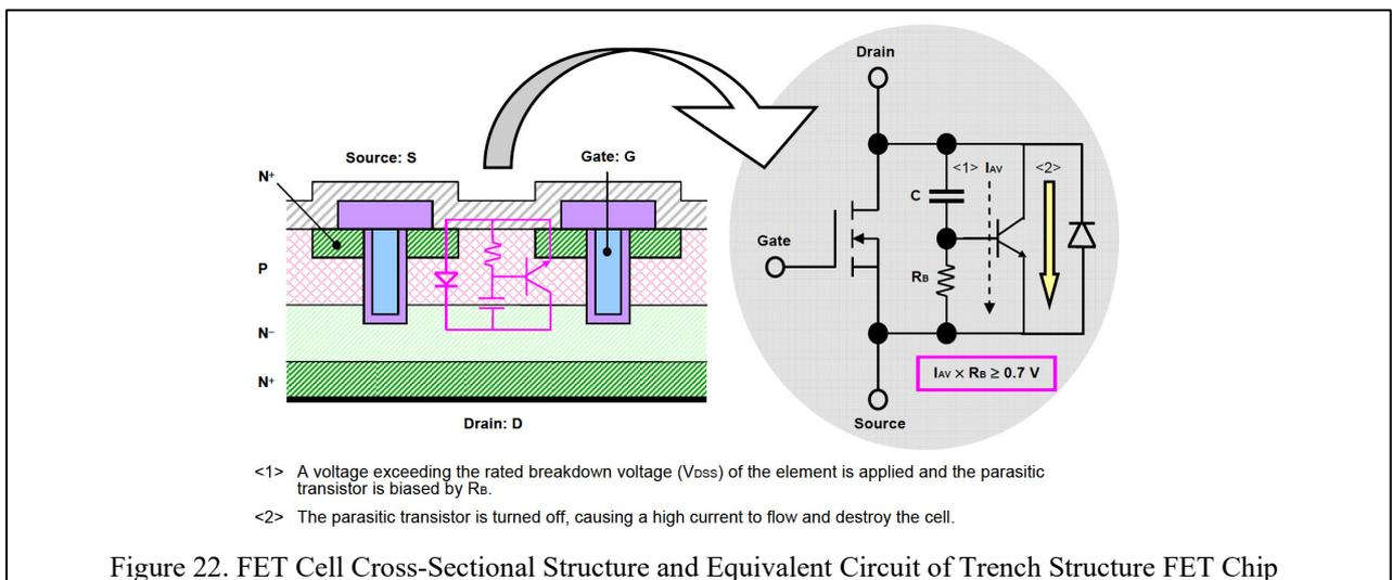
Figure 22. FET Cell Cross-Sectional Structure and Equivalent Circuit of Trench Structure FET Chip
