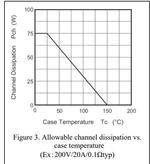
Figure 3. Allowable channel dissipation vs. case temperature (Ex: 200V/20A/0.1Ωtyp)
