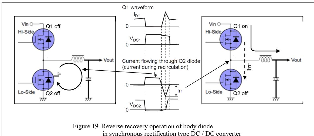
3.6.3 Body Diode Destruction Mechanism
