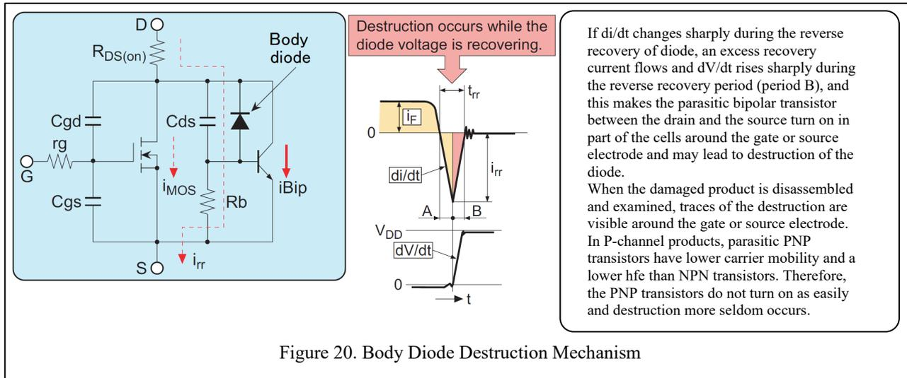
Figure 20. Body Diode Destruction Mechanism
