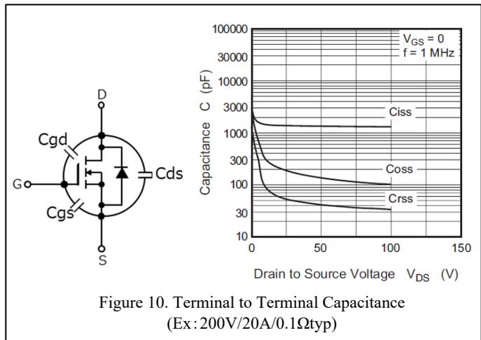
Figure 10. Terminal to Terminal Capacitance (Ex: 200V/20A/0.1Ωtyp)
