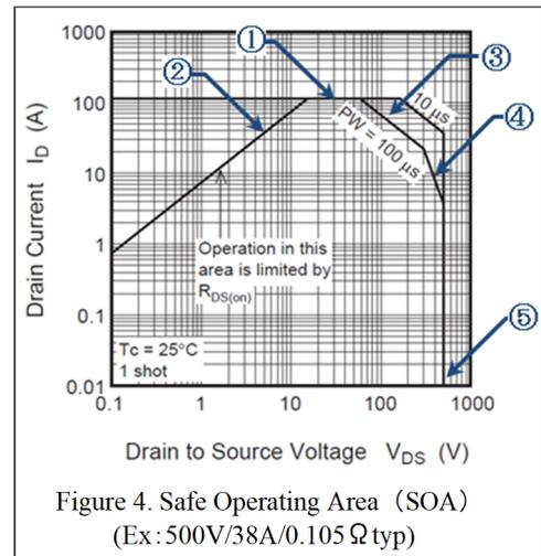
Figure 4. Safe Operating Area (SOA) (Ex: 500V/38A/0.105 Ω typ)
