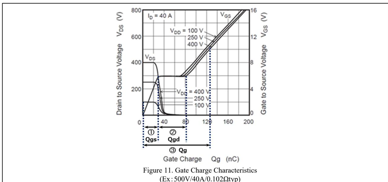
Figure 11. Gate Charge Characteristics (Ex: 500V/40A/0.102Ωtyp)
