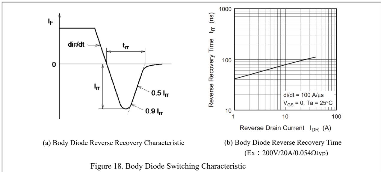
Figure 18. Body Diode Switching Characteristic
