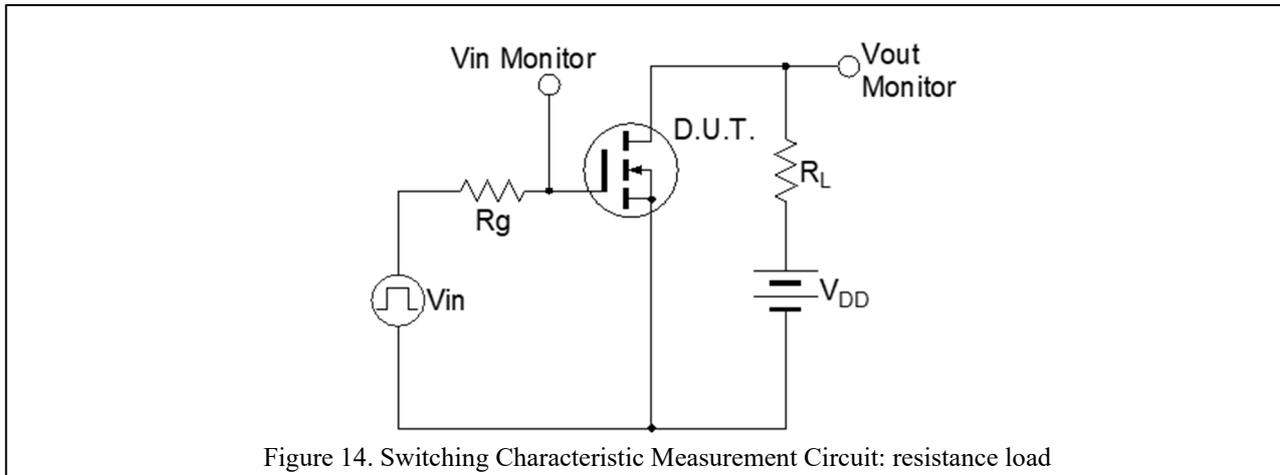
Figure 14. Switching Characteristic Measurement Circuit: resistance load
