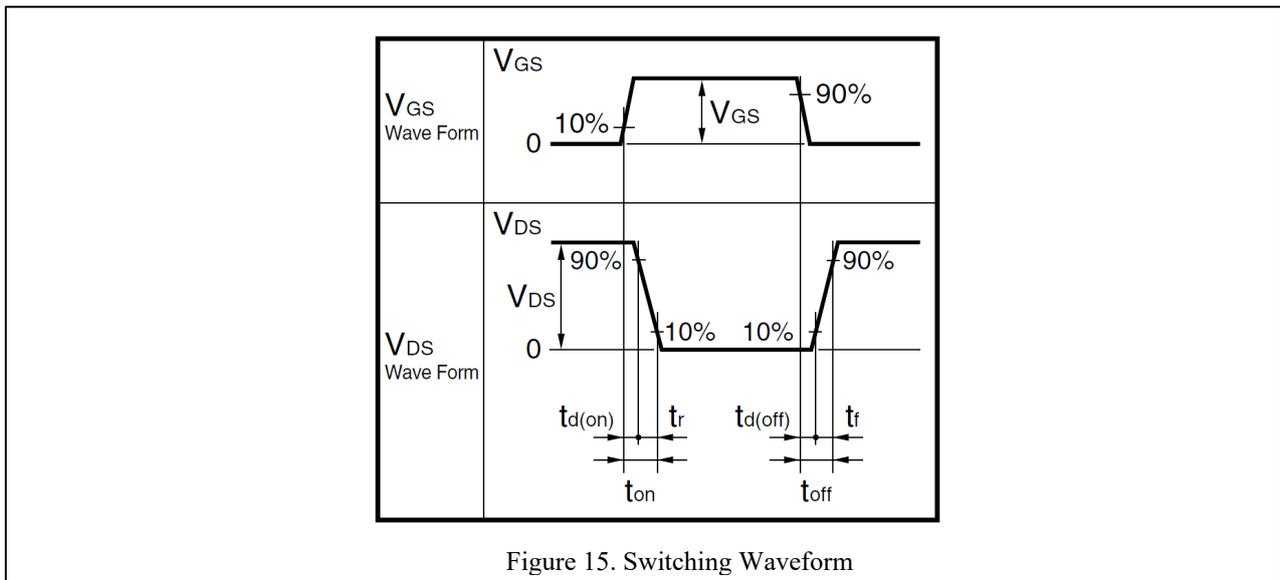
Figure 15. Switching Waveform
