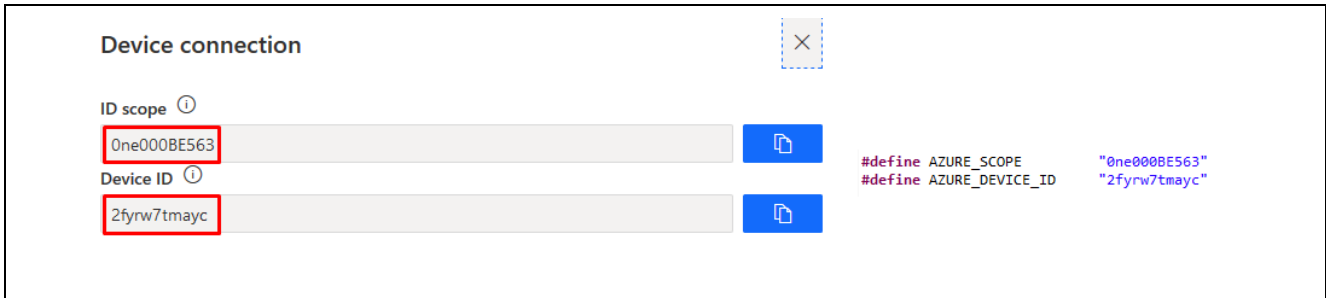
Figure 30. Device Connection Information
