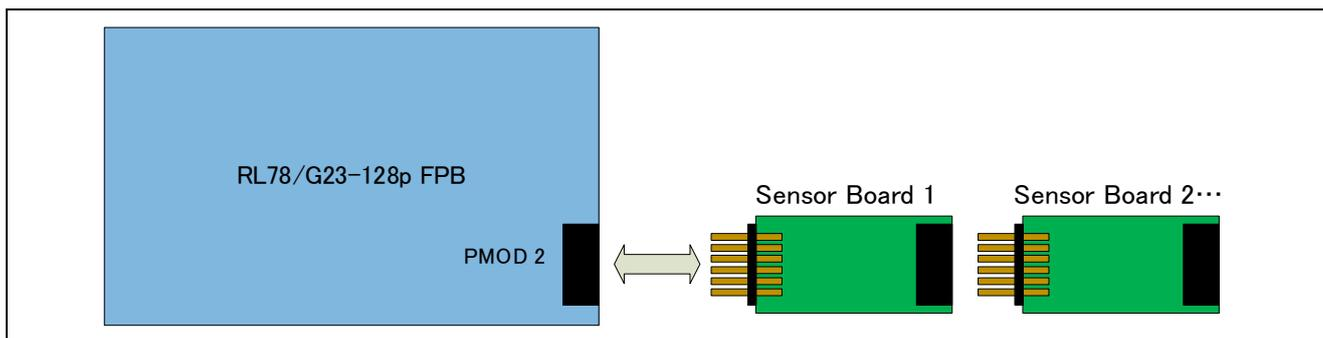
**Figure 2-5 Hardware Connections for RL78/G23-128p FPB**
