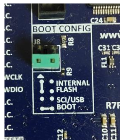
Figure 2-1 Setting J8 Jumper to 'SCI/USB BOOT' (Set When Writing FW)
