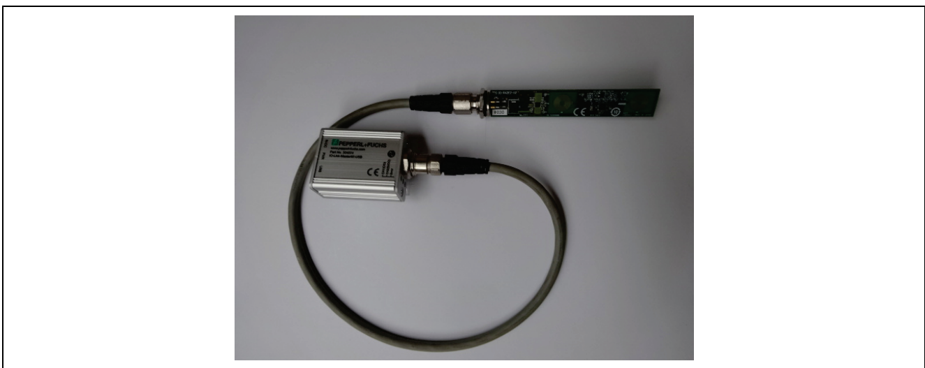
Figure 20. USB master and Inductive Sensor Board Connection
