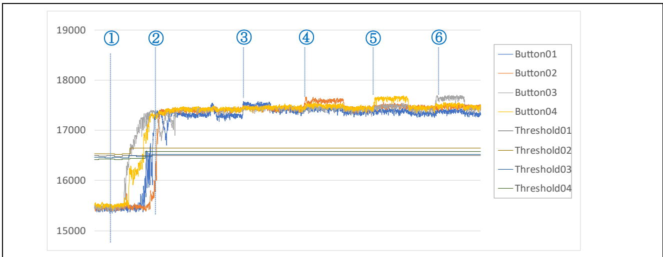
Figure 3-2 Count Value Waveform When Water Droplet Adheres to GND Shield Buttons
