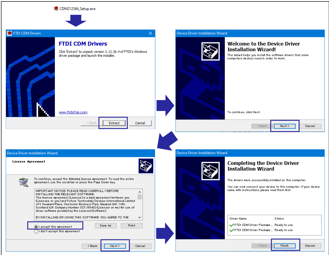
Figure 4-25 Installation of VCP driver
