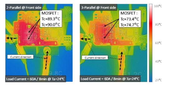
Figure 3-6 Thermograph Photo compare between 2-Parallel & 3-Parallel
