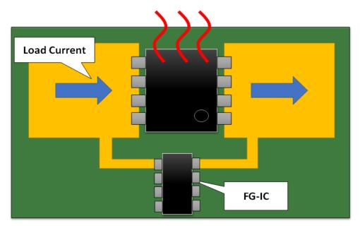
Figure 2-3 New method for MOSFET temperature monitoring
