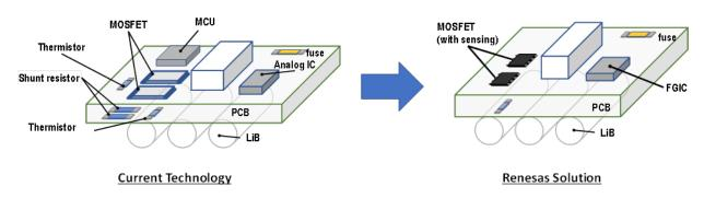
Figure 2-4 Shunt-less solution by kits of MOSFET with sensing and FGIC
