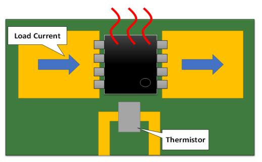
Figure 2-2 Traditional method for MOSFET temperature monitoring
