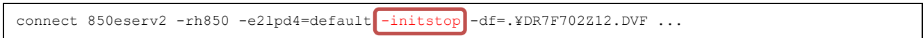
Figure 3-2 Setting for Debugging Devices with Cores in the Initially Stopped State and Operation Including Transitions to Standby Mode in MULTI
