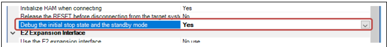
Figure 3-1 Setting for Debugging Devices with Cores in the Initially Stopped State and Operation Including Transitions to Standby Mode in CS+
