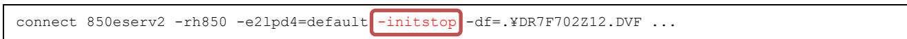
Figure 3-2 Setting for Debugging Devices with Cores in the Initially Stopped State and Operation Including Transitions to Standby Mode in MULTI
