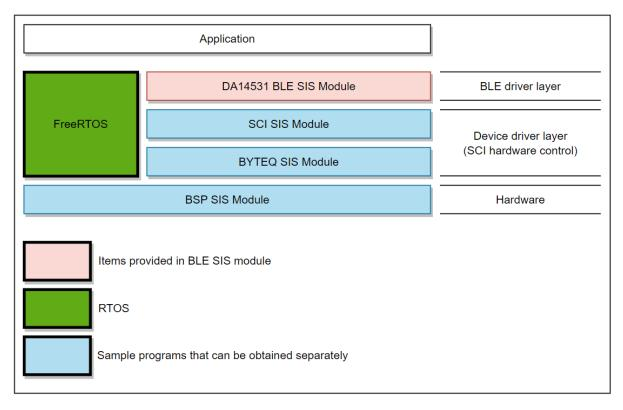
Figure 1.2 Software Configuration Diagram
