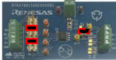
Figure 4-5 RTKA788152DE0000BU jumper pin connection picture
