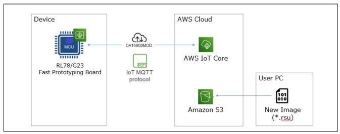
Figure 2-2 System Configuration of Demo Project (OTA)
