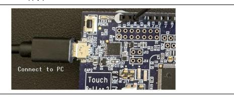
Figure 4-6 Supplying Power to the MCU Board
