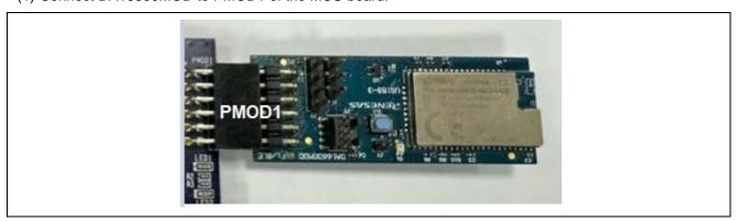
Figure 4-2 Connecting DA16600MOD to PMOD1 of the MCU Board
