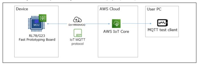
Figure 2-1 System Configuration of Demo Project (PubSub)
