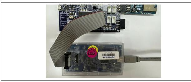
Figure 8-5 Connecting Emulator to MCU Board
