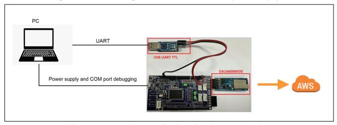
Figure 4-1 Overall Hardware Configuration of the Demo Project
