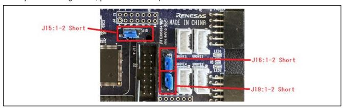
Figure 4-5 Settings for Using COM Port Debugging (Top Side)
