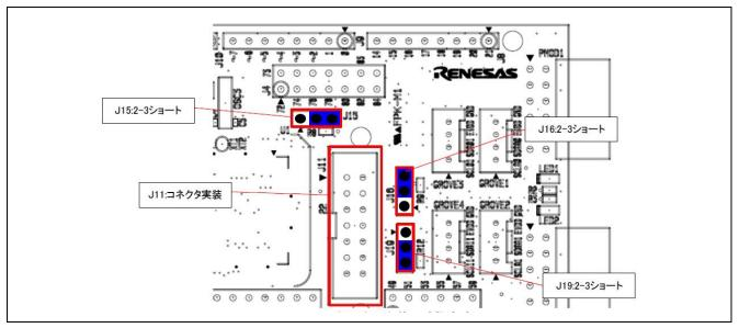
Figure 7-6 Settings for Using Emulator Connector (Top Side)
