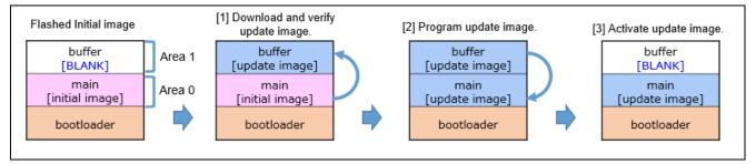
Figure 3-1 Firmware Update Mechanism
