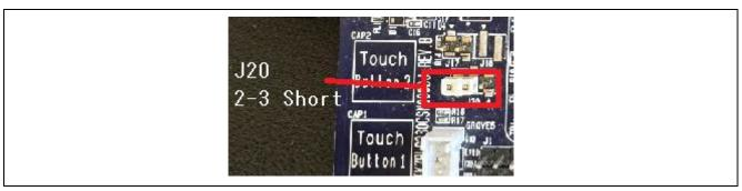
Figure 4-4 Setting MCU Board Power Supply to 3.3 V
