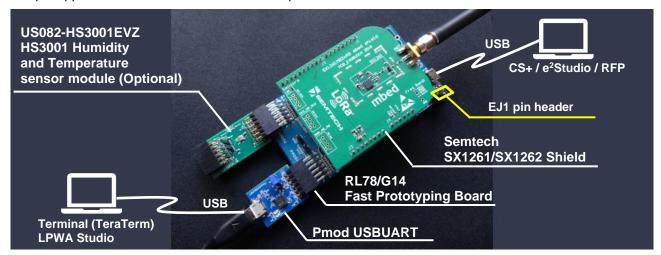
Note1: For Flash Programming or Debugging with IDE(CS+/e²studio), EJ1 pin header should be OPEN.
