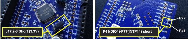
Note1: Power supply selection header (J17: default 5V) should be changed to 3.3V(J17 2-3 short).
