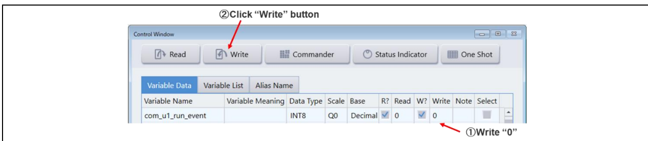
Figure 4-3 Procedure - Stop the motor
