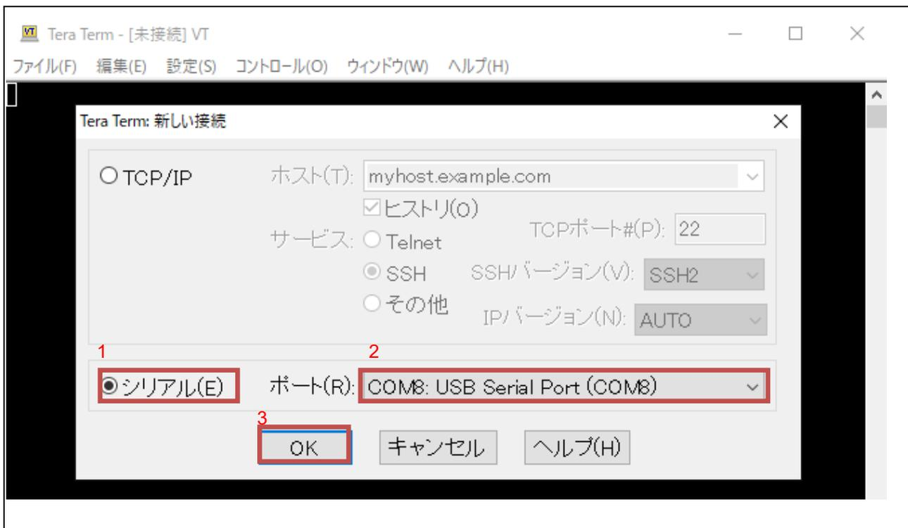
Figure 1-4 Starting TeraTerm and Port Configuration
