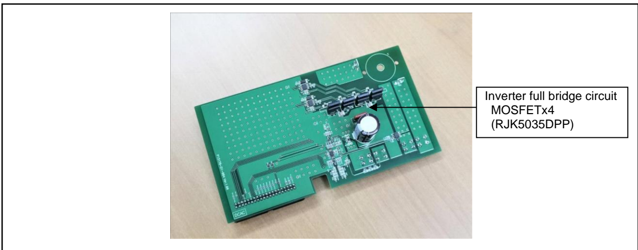
Figure 25 External view of DC-AC board
