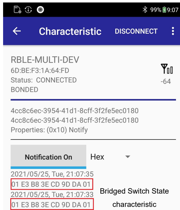
Figure 12-11 Bridged Switch State characteristic notification to central device
