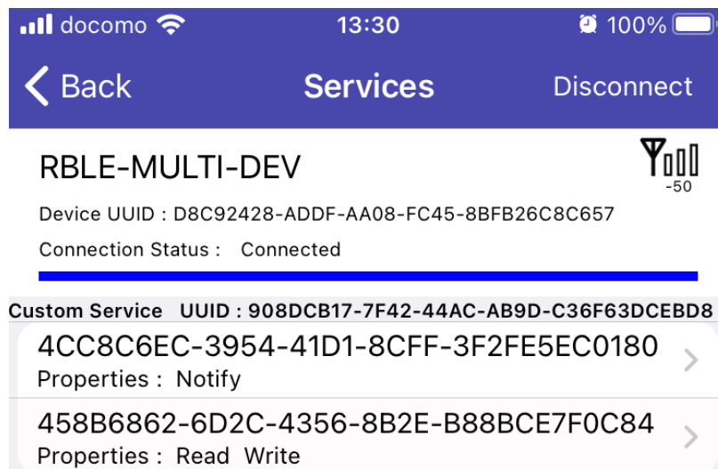
Figure 12-10 Detected GATT service and characteristics
