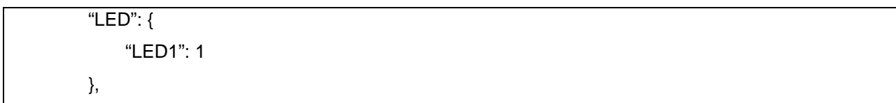
Figure 4.2 Message payload to turn on LED1
