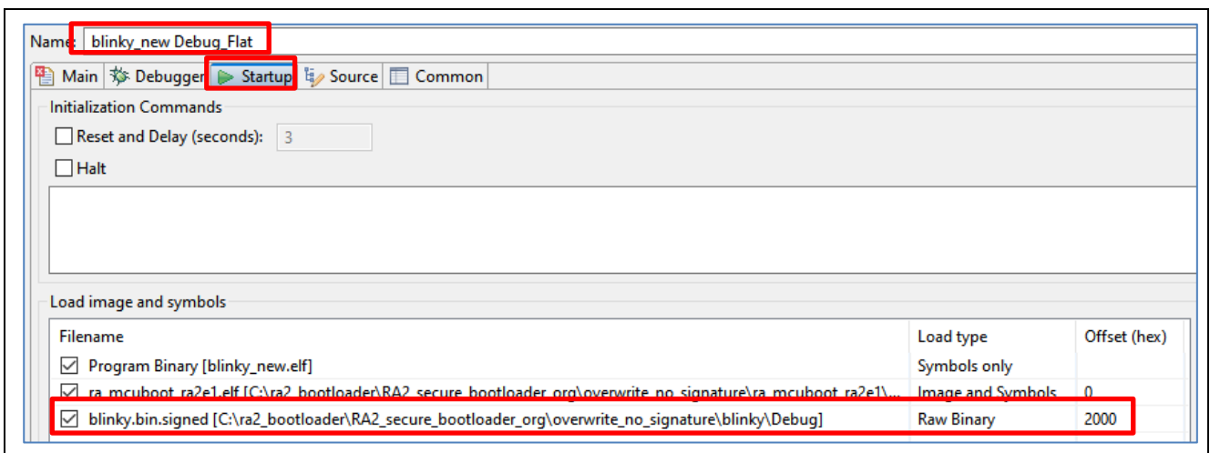
Figure 67. Debug Configuration of blinky_new initially imported
