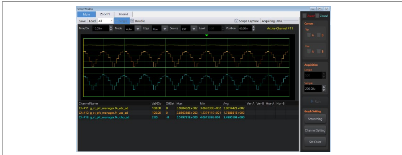
Figure 12-1 Waveforms in the State Where the Voltage is Rising Up to 390 V under PFC Control
