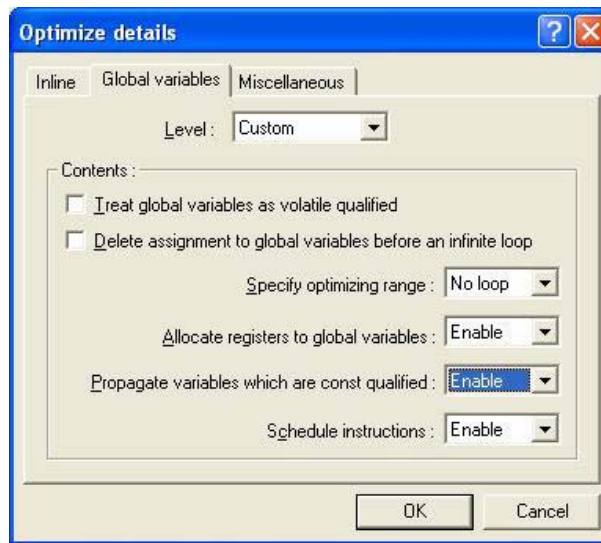
Figure 6.10 Volatile Specification for a Variable to be Shared in Tasks and Interrupts
