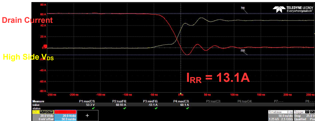
Figure 4-10 High Side Turn Off Reverse Recovery Current Waveform
