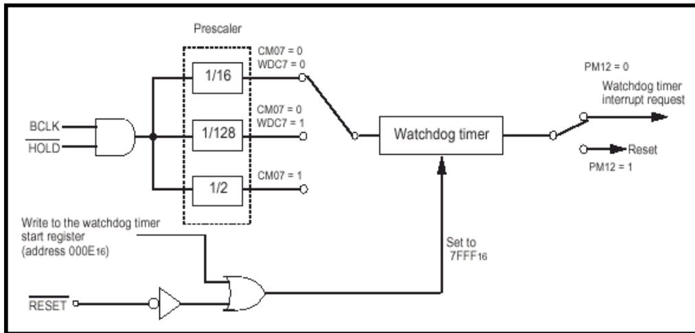
Figure 1 Watchdog Timer Block Diagram
