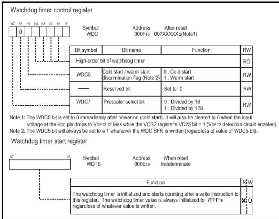
Figure 3 Watchdog Timer control and start registers
