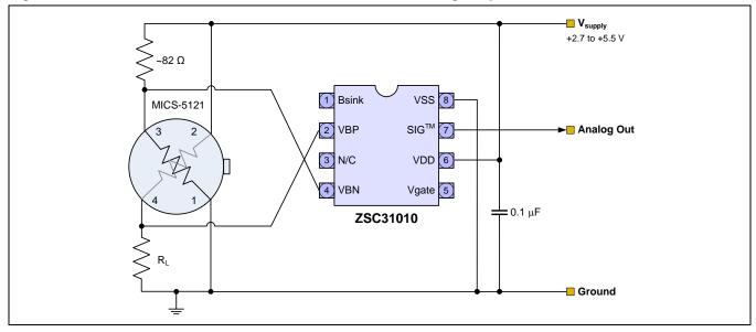
Figure 3.1 Gas Sensor Connected to the ZSC31010 with Analog Output
