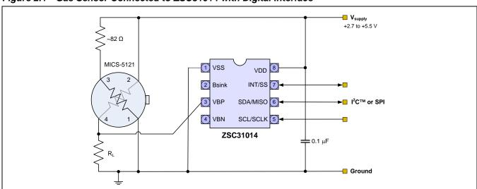
Figure 2.1 Gas Sensor Connected to ZSC31014 with Digital Interface
