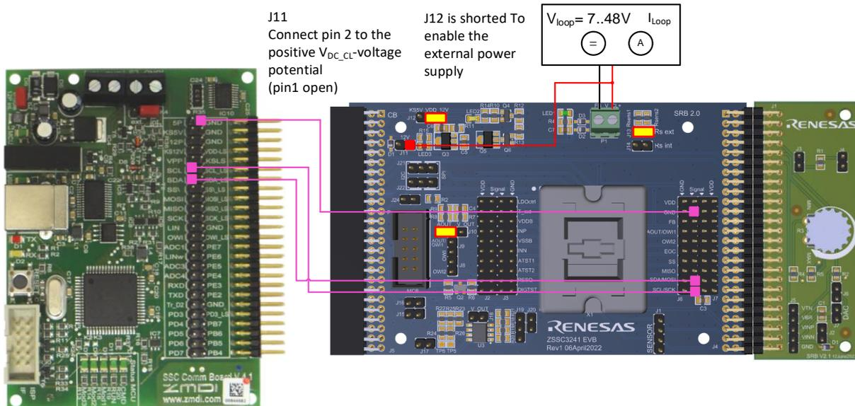
Figure 3. Current Loop HW Calibration Setup
