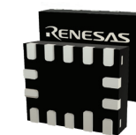
1.6 mm x 2.0 mm 14-pin STQFN 0.4 mm pitch
