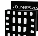
2.0 mm x 2.2 mm 22-pin MSTQFN 0.4 mm pitch
