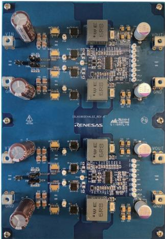
Evaluation Board with 2 cascaded ISL81802 (4-phase), 12V/40A Output
