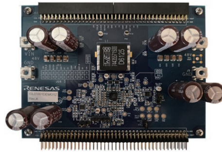
ISL81801 Evaluation Board, 80V Bi-Directional Buck-Boost controller with Current Sharing
