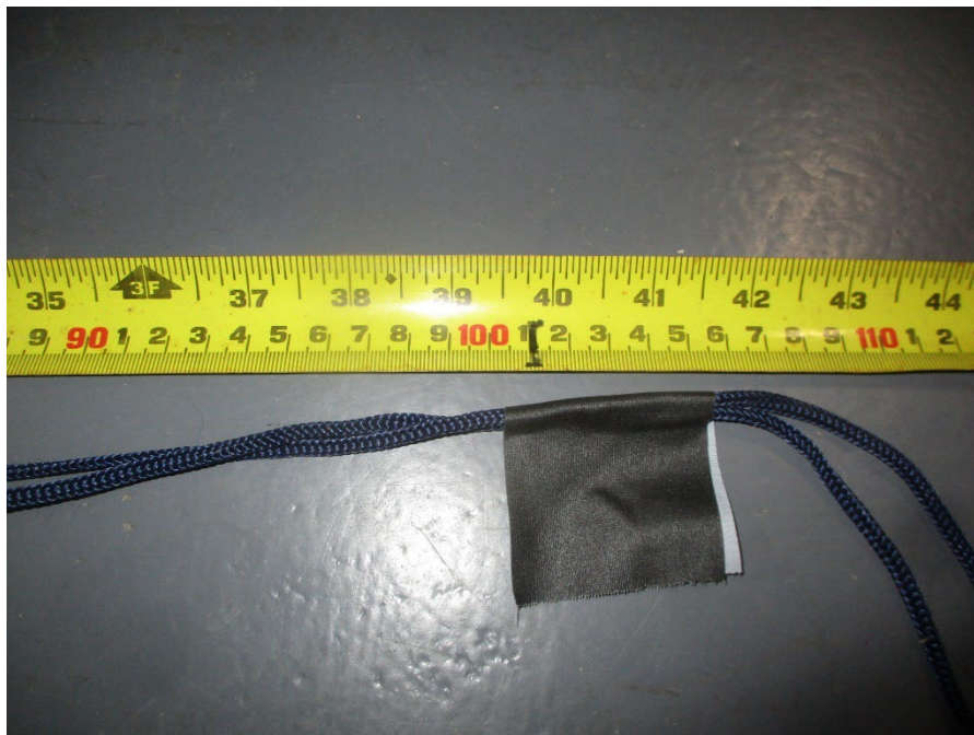
Photo 10 – Depth verification 1 meter
