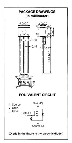
The diode connected between the gate and source of the transistor serves as a protector against ESD. When this device is actually used, an additional protection circuit is externally required if a voltage exceeding the rated voltage may be applied to this device.
