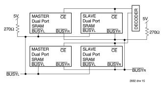
Figure 4. Busy and chip enable routing for both width and depth expansion with IDT7132 (Master) and (Slave) IDT7142 SRAMs.
