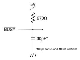
Figure 3. BUSY AC Output Test Load
