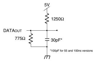
Figure 1. AC Output Test Load
