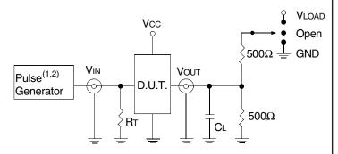
Test Circuits for All Outputs
