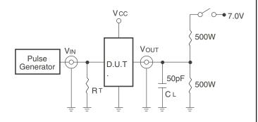
Test Circuits for All Outputs
