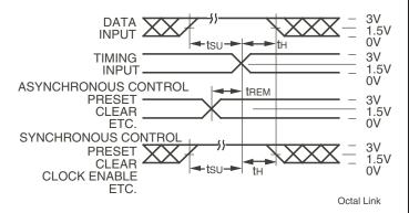
Set-Up, Hold, and Release Times
