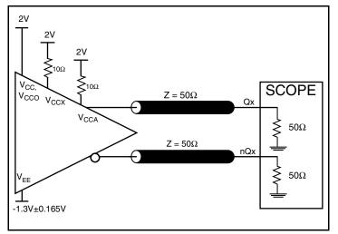
3.3V LVPECL Output Load Test Circuit
