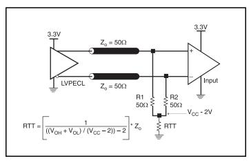
Figure 4A. 3.3V LVPECL Output Termination
