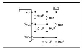
Figure 1. Power Supply Filtering
