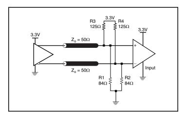
Figure 4B. 3.3V LVPECL Output Termination
