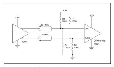
Figure 3F. CLK/nCLK Input Driven by a 2.5V SSTL Driver
