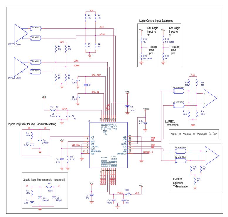
Figure 6. 813N252I-09 Application Schematic
