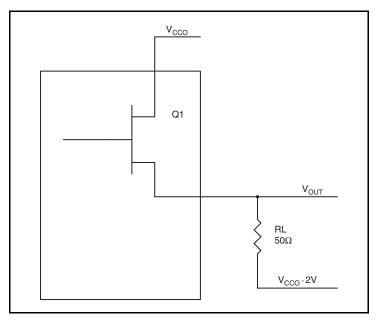
Figure 7. LVPECL Driver Circuit and Termination
