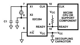
FIGURE 4. RECOMMENDED CRYSTAL AND READY CONDITIONS
