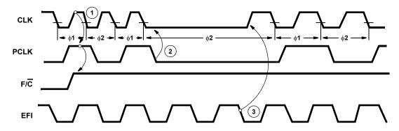
FIGURE 1B. F/C SWITCHED FROM LOW (USING THE CRYSTAL INPUT X1) TO HIGH (USING THE EFI INPUT)
