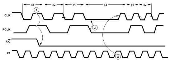
FIGURE 1A. FIC SWITCHED FROM HIGH (USING EFI INPUT) TO LOW (USING THE CRYSTAL INPUT X1)
