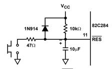
FIGURE 3. TYPICAL RC RES TIMING CIRCUIT
