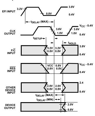
FIGURE 7. A.C. DRIVE, SETUP, HOLD AND DELAY TIME MEASUREMENT POINTS
