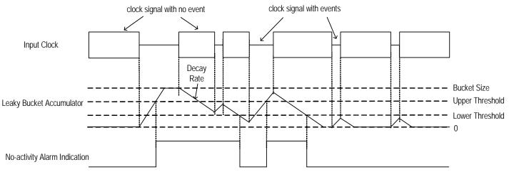
Figure 9. Input Clock Activity Monitoring
