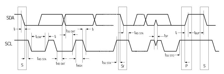
Figure 15. Definition of I2C Bus Timing
