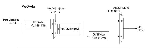
Figure 8. Pre-divider for an input clock
