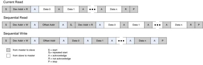
Figure 16. I2C Slave Interface Supported Transactions
