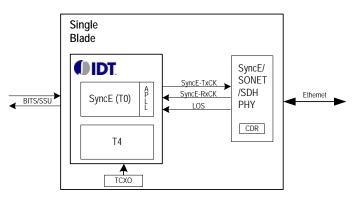
Figure 3. SyncE/SONET/SDH single blade application
