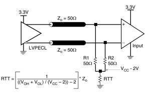
Figure 25. 3.3V LVPECL Output Termination
