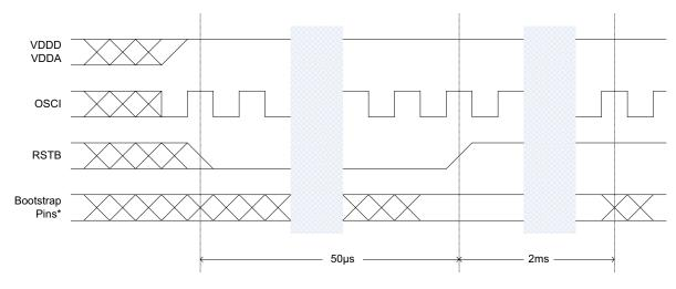
\* Bootstrap pins are: XO\_FREQ[2:0], MPU\_MODE[1:0], I2C\_AD[2:1], MS/SL, SONET/SDH
