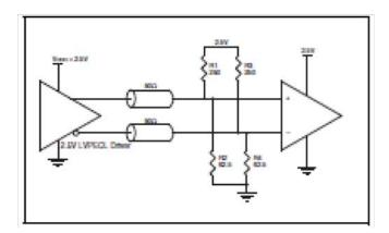
Figure 26. 2.5V LVPECL Output Termination
