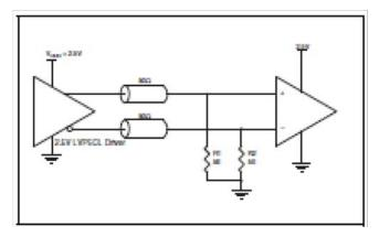
Figure 28. 2.5V LVPECL Output Termination
