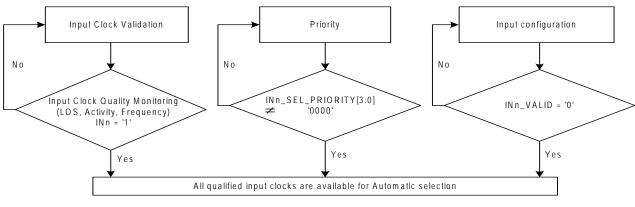
Figure 11. Qualified Input Clocks for Automatic Selection
