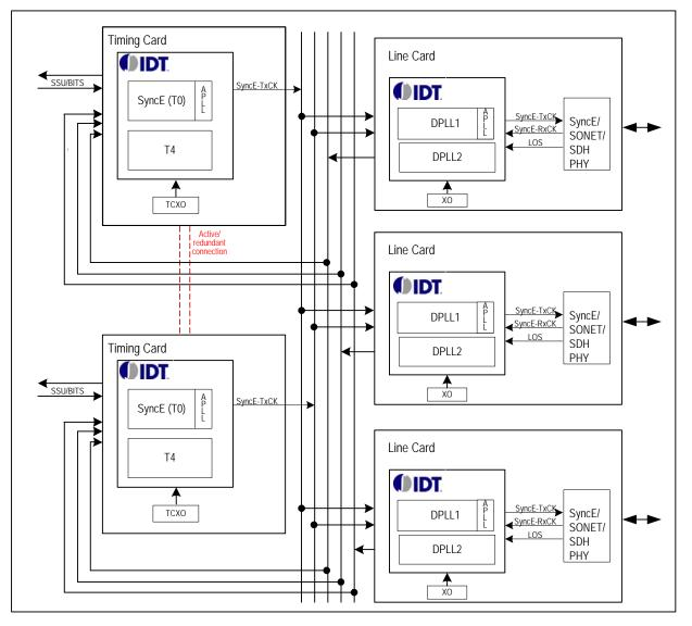
Figure 4. SyncE/SONET/SDH active/redundant application
