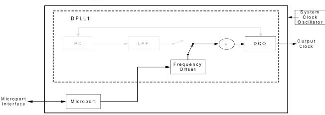
Figure 6. DCO frequency offset control functional block diagram
