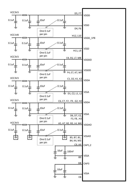
Figure 14. 82P33731 Power Decoupling Scheme
