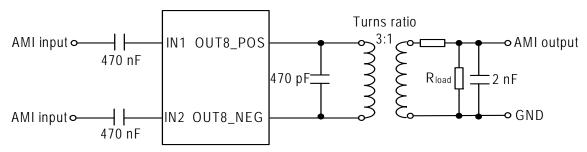
For a transformer with a turns ratio of 1:1, a 3:1 ratio potential divider R<sub>load</sub> must be used to achieve the required 1 V pk-pk voltage level for the positive and negative pulses.
