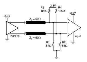
Figure 24. 3.3V LVPECL Output Termination
