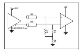
Figure 27. 2.5V LVPECL Output Termination
