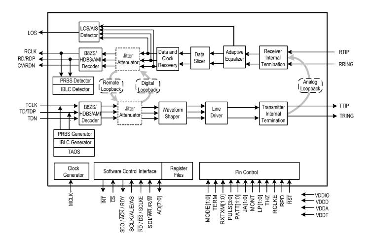
Figure-1 Block Diagram
