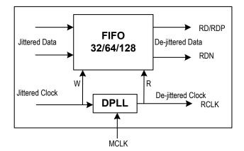
Figure-11 Jitter Attenuator
