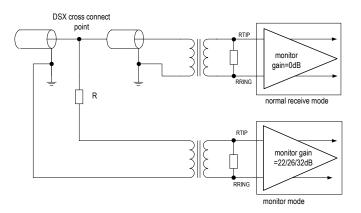
Figure-9 Monitoring Receive Line in Another Chip
