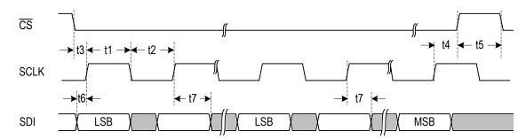
Figure-26 Serial Interface Write Timing
