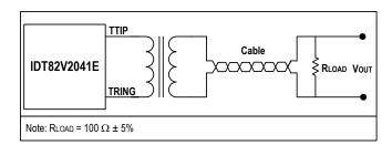
Figure-6 T1 Pulse Template Test Circuit
