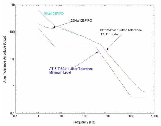
Figure-23 T1/J1 Jitter Tolerance Performance
