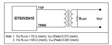
Figure-4 E1 Pulse Template Test Circuit
