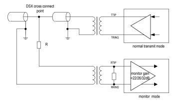
Figure-10 Monitor Transmit Line in Another Chip
