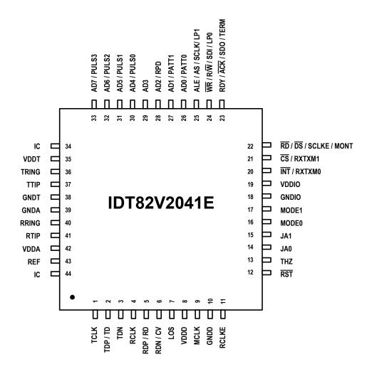
Figure-2 IDT82V2041E TQFP44 Package Pin Assignment
