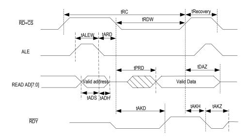
Figure-31 Multiplexed Intel Read Timing
