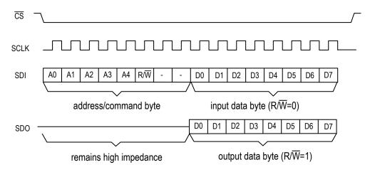
Figure-19 Serial Microcontroller Interface Function Timing
