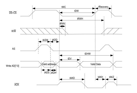
Figure-30 Multiplexed Motorola Write Timing
