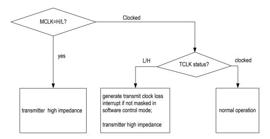
Figure-18 TCLK Operation Flowchart
