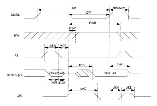
Figure-29 Multiplexed Motorola Read Timing
