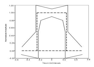
Figure-3 E1 Waveform Template Diagram
