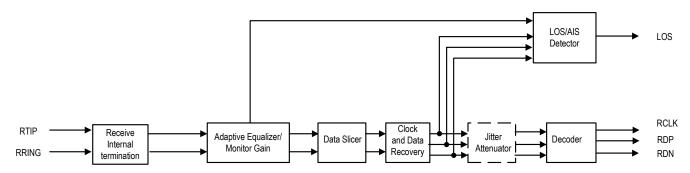
Figure-7 Receive Monitor Gain Adaptive Equalizer
