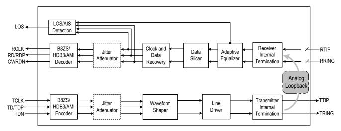
Figure-13 Analog Loopback
