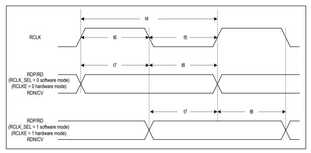
Figure-21 Receive System Interface Timing
