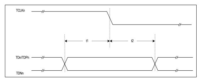
Figure-21 Transmit System Interface Timing
