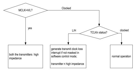
Figure-17 TCLK Operation Flowchart
