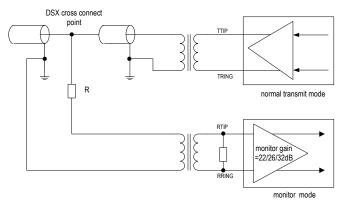
Figure-8 Monitor Transmit Line in Another Chip
