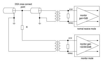
Figure-7 Monitoring Receive Line in Another Chip
