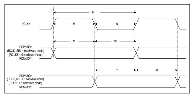
Figure-22 Receive System Interface Timing
