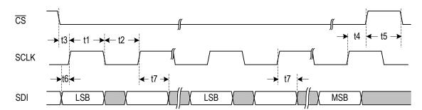
Figure-26 Serial Interface Write Timing
