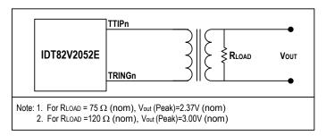
Figure-4 E1 Pulse Template Test Circuit
