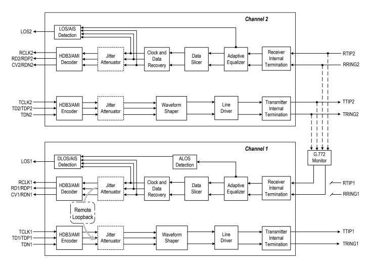
Figure-9 G.772 Monitoring Diagram
