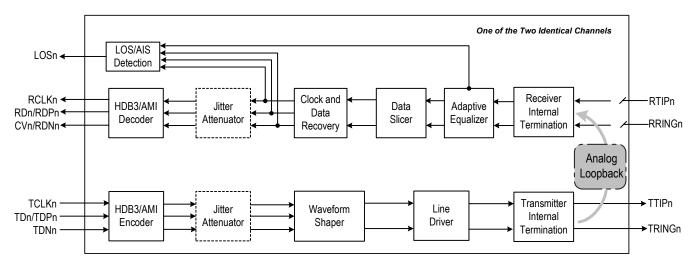
Figure-12 Analog Loopback
