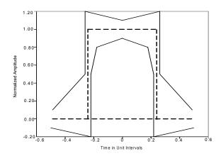
Figure-3 E1 Waveform Template Diagram
