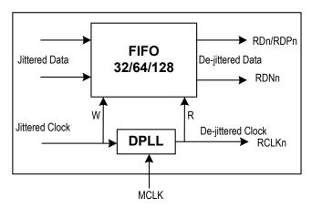
Figure-10 Jitter Attenuator
