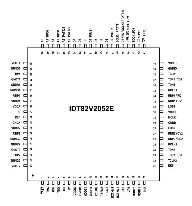
Figure-2 IDT82V2052E TQFP80 Package Pin Assignment
