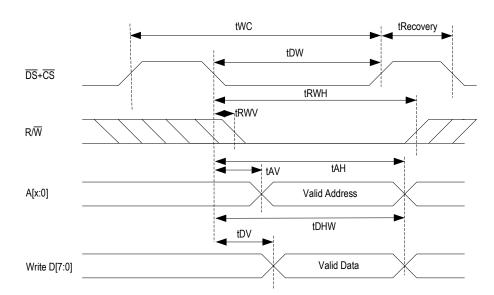
Figure-30 Non-Multiplexed Motorola Write Timing
