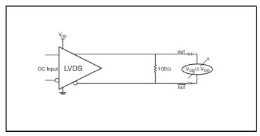
**Differential Output Voltage Setup**
