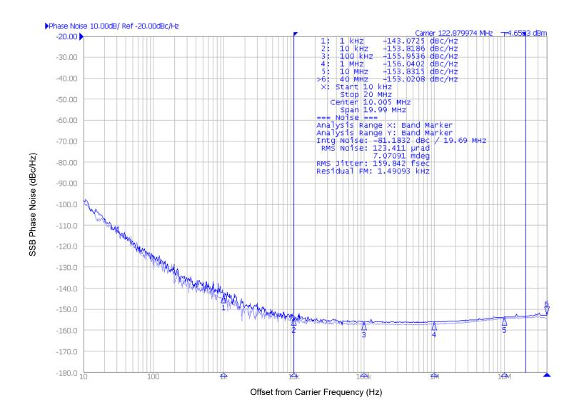
As with most timing specifications, phase noise measurements have issues relating to the limitations of the measurement equipment. The noise floor of the equipment can be higher or lower than the noise floor of the device. Additive phase noise is dependent on both the noise floor of the input source and measurement equipment.
