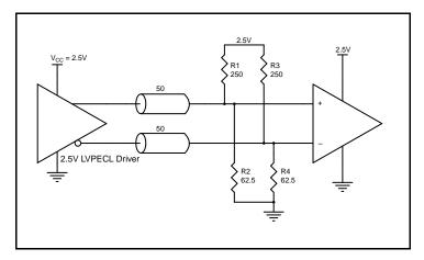
Figure 6A. 2.5V LVPECL Driver Termination Example
