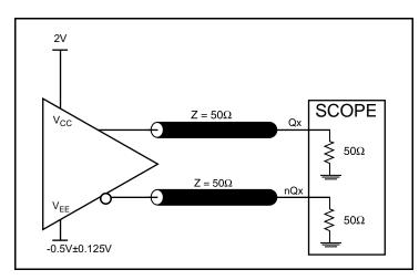
2.5V LVPECL Output Load AC Test Circuit
