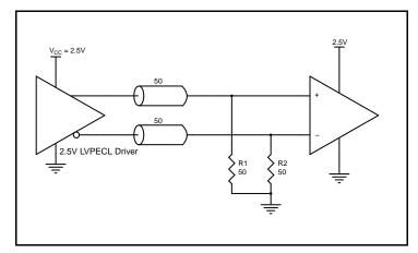
Figure 6C. 2.5V LVPECL Driver Termination Example
