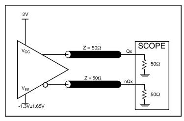
3.3V LVPECL Output Load AC Test Circuit
