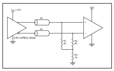
Figure 6B. 2.5V LVPECL Driver Termination Example
