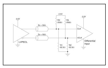
Figure 4A. CLK/nCLK Input Driven by a 2.5V LVPECL Driver
