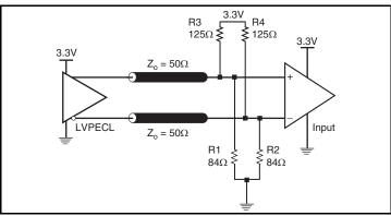
Figure 6B. 3.3V LVPECL Output Termination
