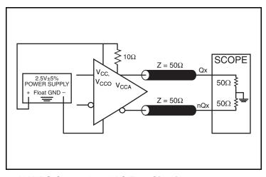
2.5V LVDS Output Load AC Test Circuit
