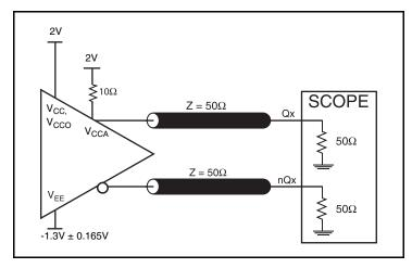
3.3V LVPECL Output Load AC Test Circuit
