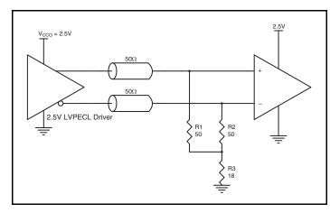
Figure 7B. 2.5V LVPECL Driver Termination Example
