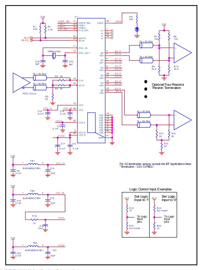
Figure 9. IDT8T49N006I Application Schematic
