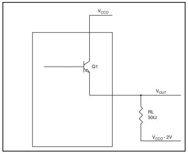
Figure 10. LVPECL Driver Circuit and Termination
