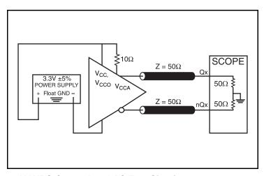
3.3V LVDS Output Load AC Test Circuit
