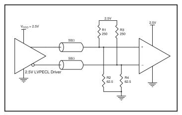
Figure 7A. 2.5V LVPECL Driver Termination Example
