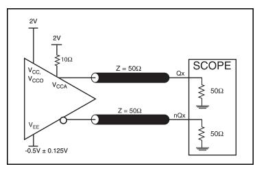
2.5V LVPECL Output Load AC Test Circuit
