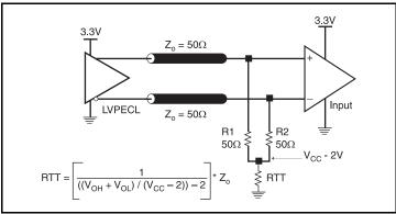
Figure 6A. 3.3V LVPECL Output Termination
