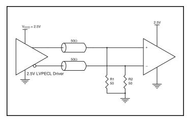
Figure 7C. 2.5V LVPECL Driver Termination Example
