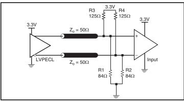
Figure 6B. 3.3V LVPECL Output Termination
