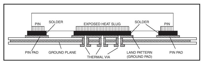
Figure 8. P.C. Assembly for Exposed Pad Thermal Release Path – Side View (drawing not to scale)
