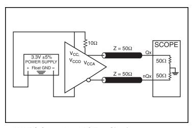
3.3V LVDS Output Load AC Test Circuit
