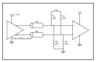
Figure 7A. 2.5V LVPECL Driver Termination Example
