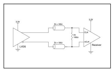
Figure 3D. CLK/nCLK Input Driven by a 3.3V LVDS Driver
