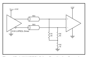
Figure 7B. 2.5V LVPECL Driver Termination Example
