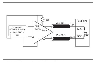
2.5V LVDS Output Load AC Test Circuit
