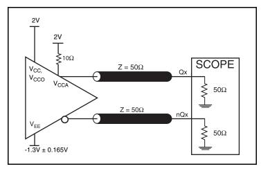
3.3V LVPECL Output Load AC Test Circuit
