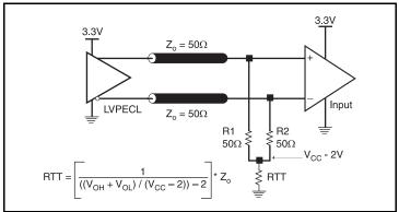
Figure 6A. 3.3V LVPECL Output Termination
