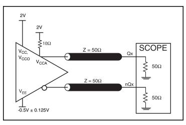
2.5V LVPECL Output Load AC Test Circuit
