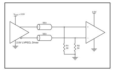
Figure 7C. 2.5V LVPECL Driver Termination Example
