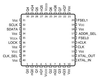
IDT8T49N008I 40-Lead VFQFN 6mm x 6mm x 0.925mm package body 4.65mm x 4.65mm E-Pad NL Package
