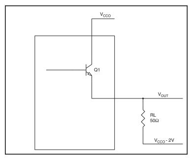
Figure 10. LVPECL Driver Circuit and Termination
