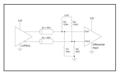
Figure 3A. CLK/nCLK Input Driven by a 3.3V LVPECL Driver
