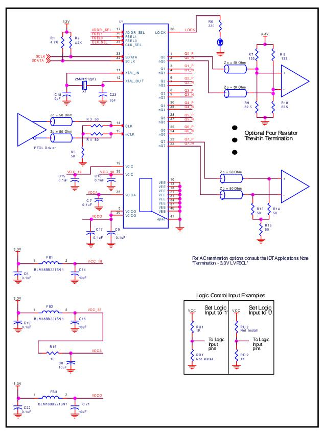
Figure 9. IDT8T49N008I Application Schematic
