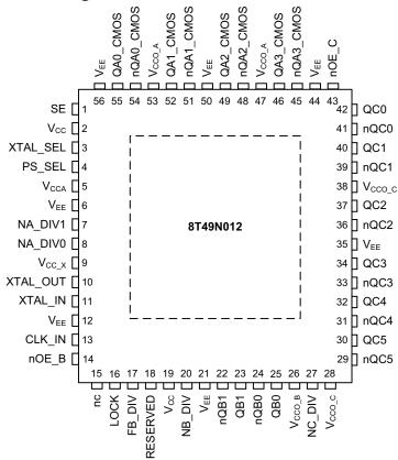
56-Lead VFQFN, 8.0mm x 8.0mm x 0.9mm
