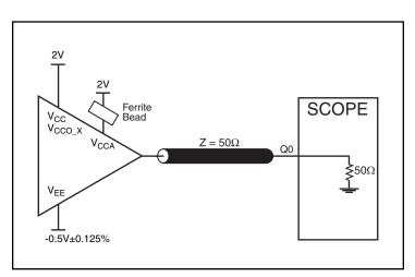
2.5V/2.5V QAx\_CMOS Output Load Test Circuit
