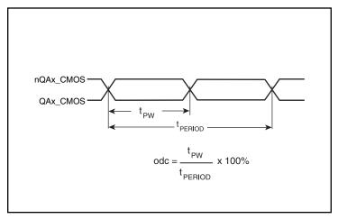
LVCMOS Output Duty Cycle/Pulse Width/Period
