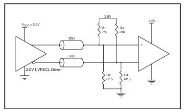
Figure 4A. 2.5V LVPECL Driver Termination Example
