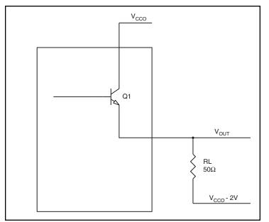
Figure 6. LVPECL Driver Circuit and Termination
