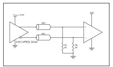
Figure 4C. 2.5V LVPECL Driver Termination Example
