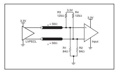
Figure 3A. 3.3V LVPECL Output Termination
