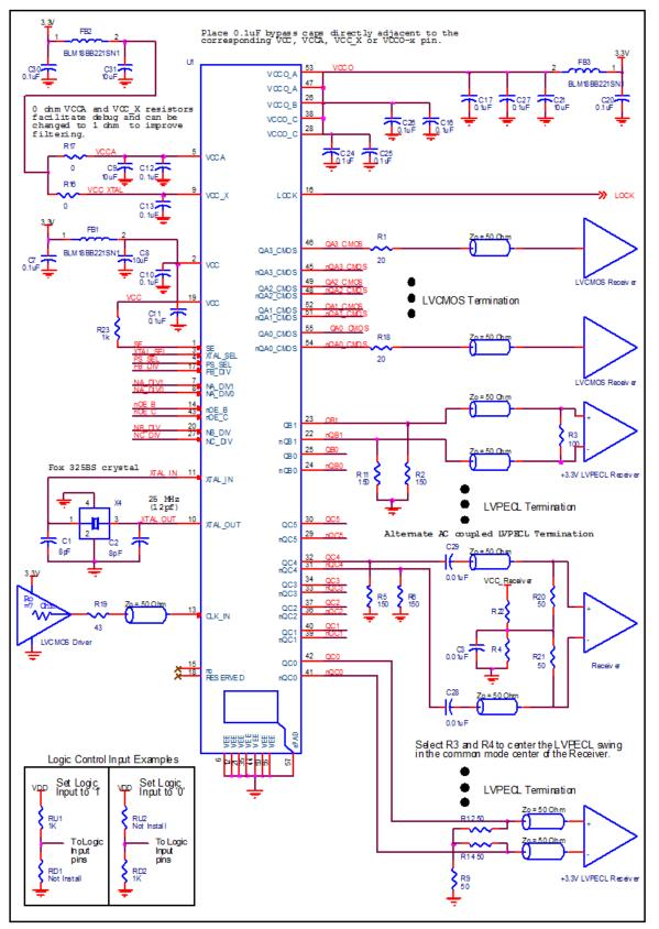
Figure 5. 8T49N012 Schematic Example
