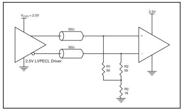
Figure 4B. 2.5V LVPECL Driver Termination Example
