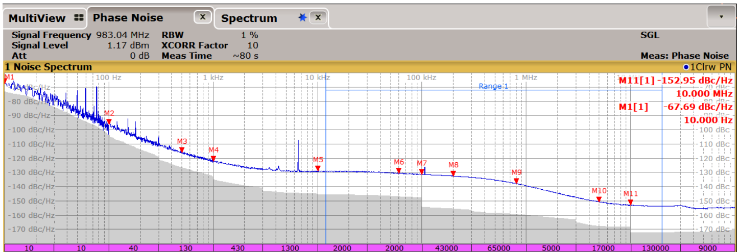
Figure 12. 983.04MHz Output Phase Noise
