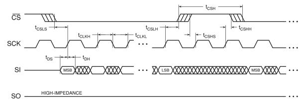
Figure 14-2. Serial Output Timing
