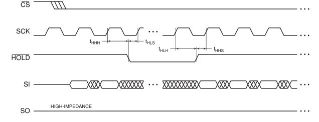
Figure 14-5. HOLD Timing – Serial Output
