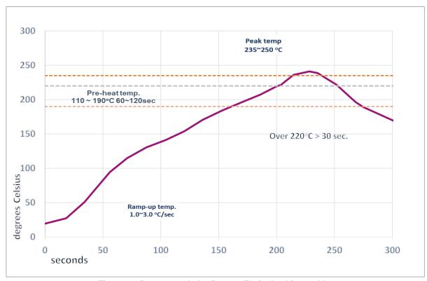
Figure 22. Recommended reflow profile for lead free solder
