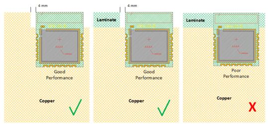
Figure 10. Antenna performance in proximity of copper (left), laminate (middle), and laminate under antenna (right)
