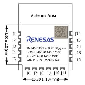
Figure 3. Module shield marking
