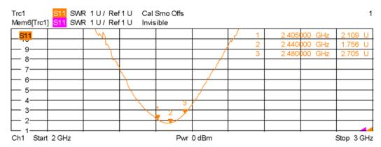
Figure 13. VSWR with module installed in center (position #2) of the evaluation board
