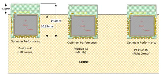
Figure 9. Installation locations for optimum antenna performance
