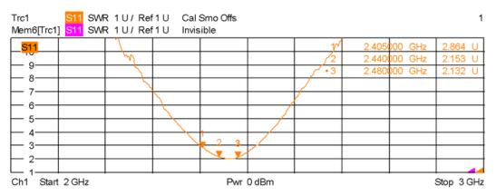
Figure 14. VSWR with module installed in upper-right corner (position #3) of the evaluation board
