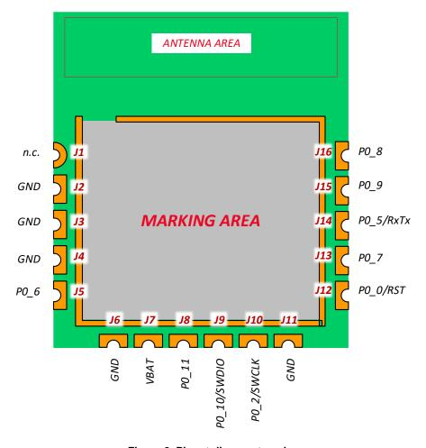
Figure 2. Pinout diagram top view
