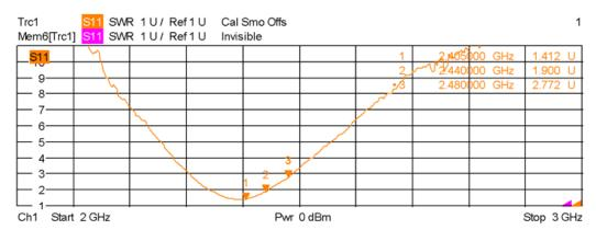
Figure 12. VSWR installed in upper-left corner (position #1) of evaluation board
