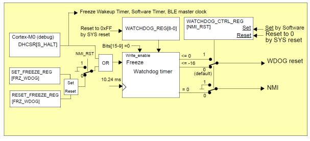
Figure 60: Watchdog Timer Block Diagram
