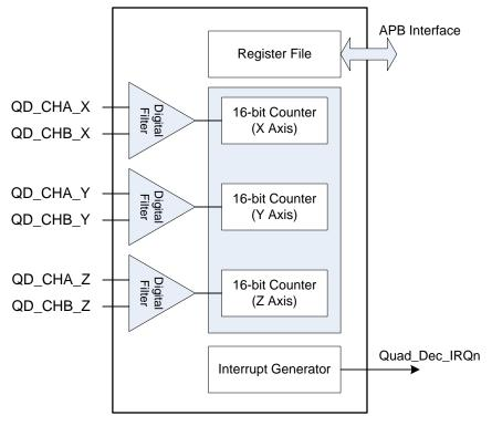
Figure 51: Quadrature Decoder Block Diagram
