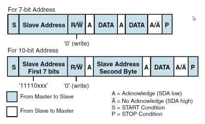
Figure 34: Master-Transmitter Protocol
