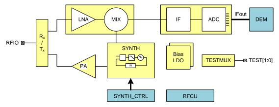
Figure 84: Bluetooth® Radio Block Diagram
