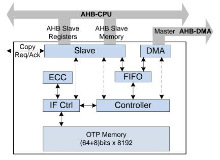
Figure 24: OTP Controller Block Diagram
