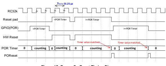
Figure 15: Power-On Reset Timing Diagram
