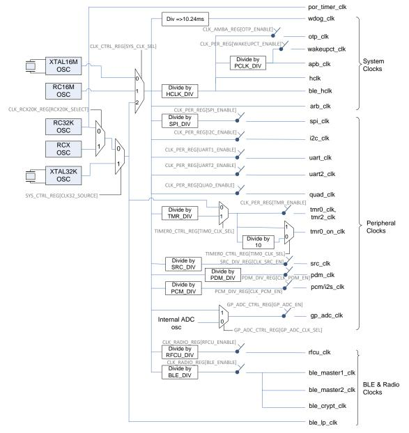
Figure 23: Clock Generation Block Diagram
