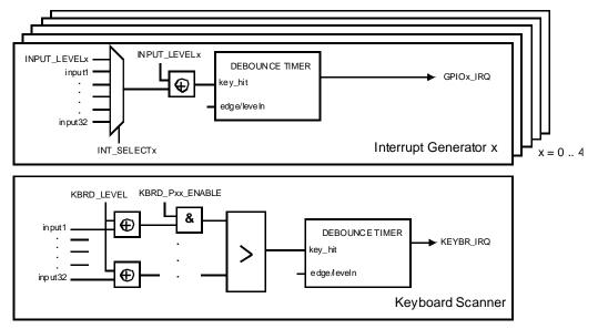
Figure 61: Keyboard Controller Block Diagram
