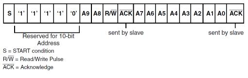
Figure 33: 10-bit Address Format
