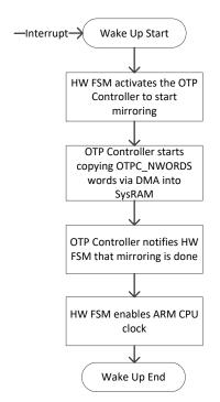
Figure 11: Wake-Up OTP Mirroring
