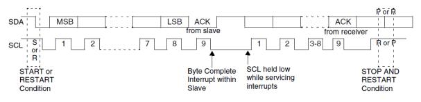
Figure 30: Data Transfer on the I2C Bus
