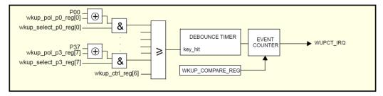
Figure 54: Wake-Up Timer Block Diagram
