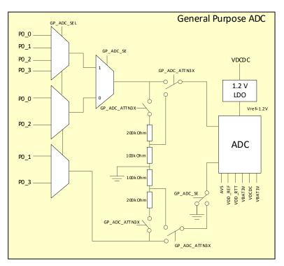
Figure 65: Block Diagram of the General-Purpose ADC
