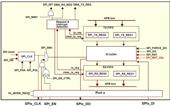
Figure 45: SPI Block Diagram
