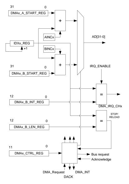
Figure 27: DMA Channel Diagram
