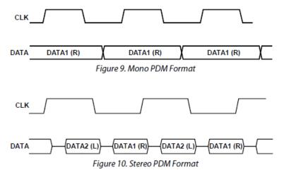
Figure 72: PDM Mono/Stereo Formats
