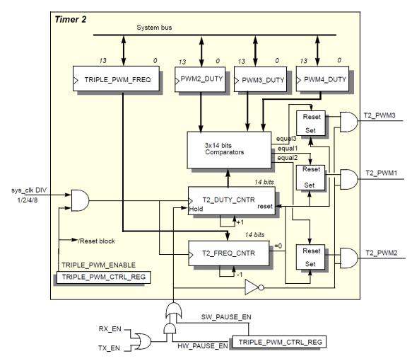
Figure 58: Timer 2 PWM Block Diagram
