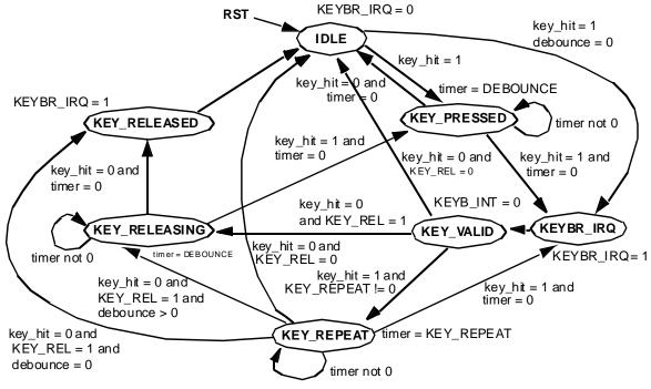
Figure 62: Keyboard Scanner State Machine
