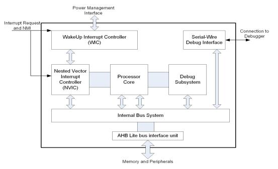
A simplified block diagram of the Cortex-M0 is shown in Figure 16.
