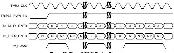
Figure 59: Timer 2 PWM Timing Diagram
