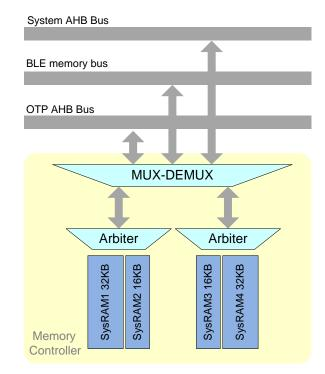
Figure 19: Memory Controller Block Diagram
