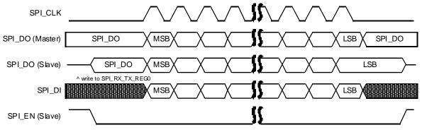
Figure 47: SPI Master/Slave, Mode 1: SPI\_POL=0 and SPI\_PHA=1
