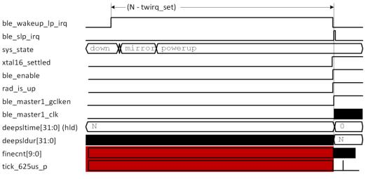
Figure 82: Exit BLE Deep Sleep Mode at Predetermined Time (Zoom Out)
