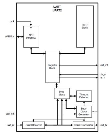
Figure 39: UART Block Diagram
