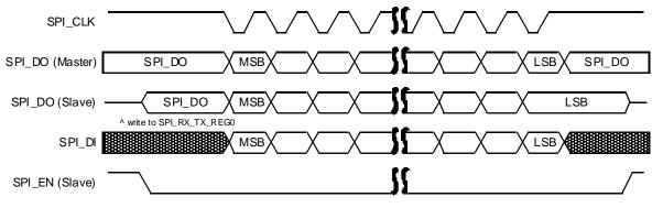
Figure 49: SPI Master/slave, Mode 3: SPI\_POL=1 and SPI\_PHA=1
