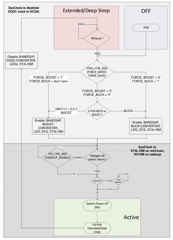
Figure 10: Power/Wake-Up Sequence
