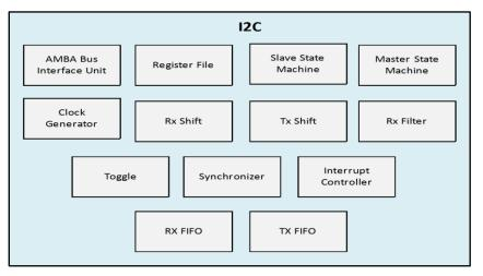
Figure 28: I2C Controller Block Diagram
