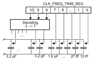
Figure 22: 16 MHz Crystal Oscillator Frequency Trimming
