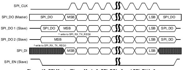
Figure 46: SPI Master/Slave, Mode 0: SPI\_POL=0 and SPI\_PHA=0
