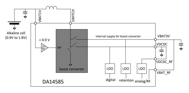
Figure 76: Supply Overview, Alkaline-Cell Application
