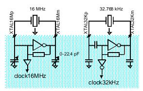
Figure 21: Crystal Oscillator Circuits
