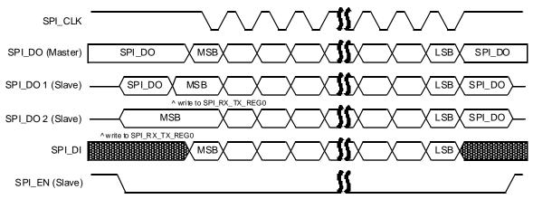
Figure 48: SPI Master/Slave, Mode 2: SPI\_POL=1 and SPI\_PHA=0
