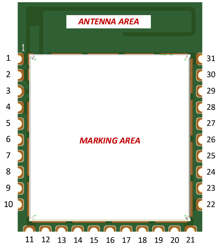
Figure 4. Pinout diagram – top view
