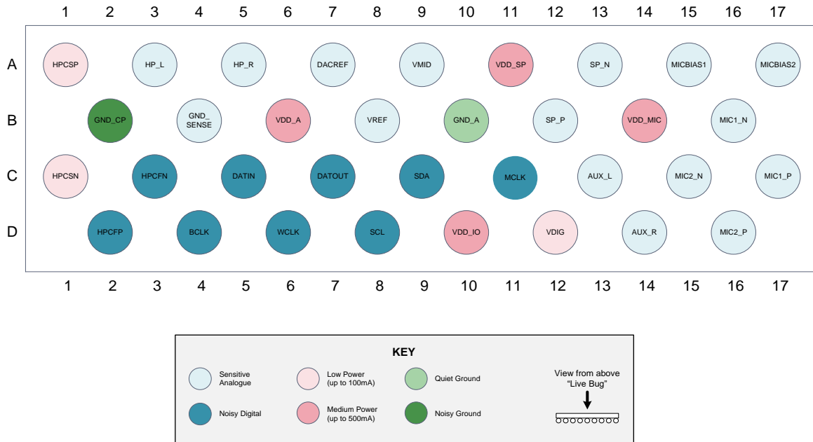
Figure 3. DA7212 ball layout
