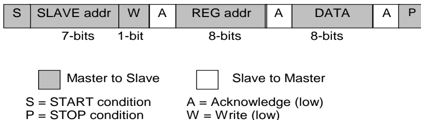
Figure 34: I 2 C Byte Write (SDA line)
