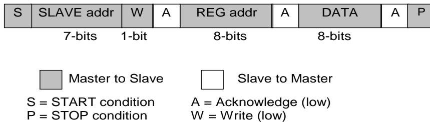
Figure 35: I 2 C Byte Write (SDA line)
